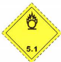
(No. 5.1) Symbol (flame over circle): black; Background: yellow; Figure '5.1' in bottom corner
