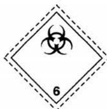
(No. 6.2) The lower half of the label may bear the inscriptions: 'INFECTIOUS SUBSTANCE' and 'In the case of damage or leakage immediately notify Public Health Authority'; Symbol (three crescents superimposed on a circle) and inscriptions: black; Background: white; Figure '6' in bottom corner
