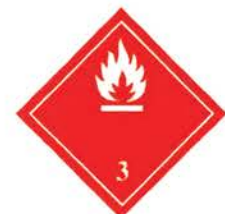
(No. 3) Symbol (flame): black or white; Background: red; Figure '3' in bottom corner
