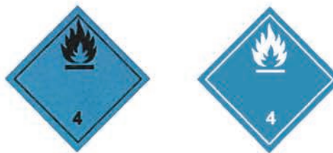
(No. 4.3) Symbol (flame): black or white; Background: blue; Figure '4' in bottom corner
